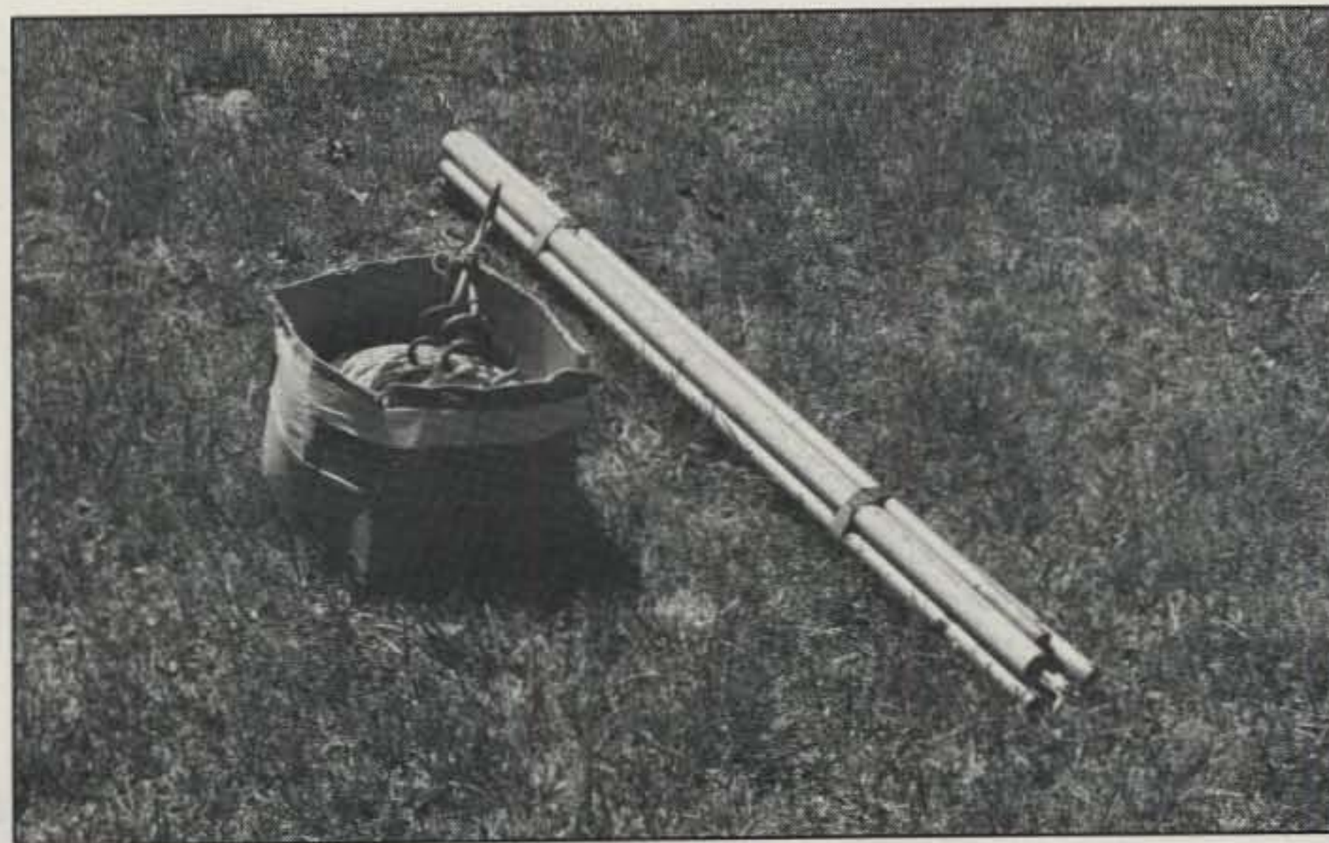
Fig. 7- The portable antenna and mast break down into a 5 foot long bundle and a small box for travel.
